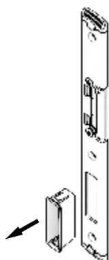
2. Install spacer (only on u-shaped strike plates)
