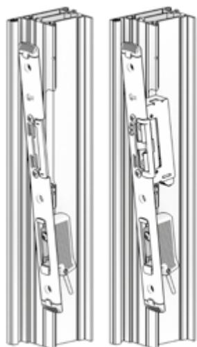
7. Depending on the deadbolt length, partially unscrew or completely remove the screw for setting the switching point (Allen key SW 2.5).
